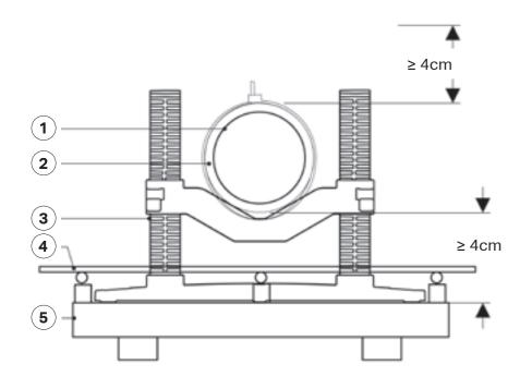
Figure 3: Embedding a Geberit cast-in concrete bracket in concrete on formwork
